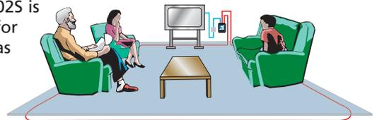
where it allows hearing aid users to enjoy TV/radio broadcasts. It includes an APS scart lead, an APL dual phono Outreach connection plate, 30m of loop cable and two 'loop in use' stickers.
