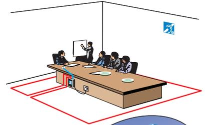
Ideal for council chambers, seminar rooms and doctors' surgeries up to 7m x 7m in size. Includes an AMT tie/desk microphone, 30m of loop cable and two 'loop in use' stickers.
